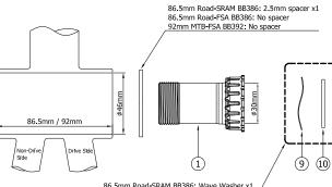
86.5mm Road-SRAM BB386: Wave Washer x1 92mm MTB-FSA BB392: 2mm spacer x1
